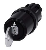
key-operated switch Siemens, 22 mm, round, plastic, lock number SSG10, with 2 keys, 3 switch positions >O<II, momentary contact on the left, latching on the right, actuating angle  $2x45^\circ$ , 10:30h/12h/13:30h, key removal O, with laser labeling, upper case and lower case, always upper case at beginning of line
