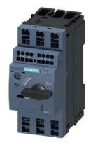
Circuit breaker size S00 for motor protection, CLASS 10 A-release 1.8...2.5 A N-release 33 A Spring-type terminal Standard switching capacity with transverse auxiliary switches 1 NO+1 NC
