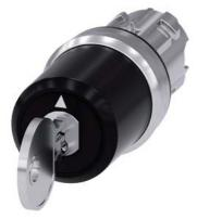
key-operated switch Siemens, 22 mm, round, metal, shiny, lock number SSG10, with 2 keys, 3 switch positions I>O<II, momentary contact type, actuating angle 2x45°, 10:30h/12h/13:30h, key removal O, with laser labeling, upper case and lower case, always upper case at the beginning of the word
