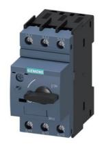
Circuit breaker size S0 for motor protection, CLASS 10 A-release 11...16 A N-release 208 A screw terminal Switching capacity 30 kA at 600 V according to UL/CSA
