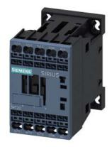
power contactor, AC-3e/AC-3, 9 A, 4 kW / 400 V, 3-pole, 24 V DC, auxiliary contacts: 1 NC, spring-loaded terminal, size: S00  $\,$
