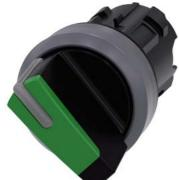
Selector switch, illuminable, 22 mm, round, plastic with metal front ring, green, selector switch, short, 2 switch positions O-I, latching, actuating angle 90°, 10:30h/13:30h, with laser labeling, upper case and lower case, always upper case at beginning of line
