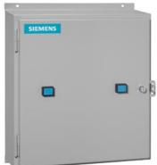
Duplex starter w/o alternator, Size 0, Three phase full voltage, Solid-state overload relay, OLR amp range 0.25-1A, 110V 50Hz / 120V 60Hz coil, Non-combination type, Enclosure NEMA type 12, Dust/drip proof for indoors
