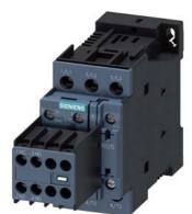
power contactor, AC-3e/AC-3, 12 A, 5.5 kW / 400 V, 3-pole, 24 V DC, auxiliary contacts: 2 NO + 2 NC, screw terminal, size: S0, removable auxiliary switch
