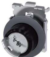
RONIS key-operated switch, 30 mm, round, Metal, matte, front ring for flush installation, lock number SB30, with 2 keys, 2 switch positions O<I, momentary contact type, Actuating angle 45°, 10:30h/12h, key removal O, possible special locks: SB31, 421, 455, with laser labeling, upper case and lower case, always upper case at beginning of line
