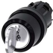
RONIS key-operated switch, 22 mm, round, plastic, lock number SB30, with 2 keys, 3 switch positions I>O-II, momentary contact on the left, latching on the right, actuating angle 2x45°, 10:30h/12h/13:30h, key removal O, possible special locks: SB31, 421, 455
