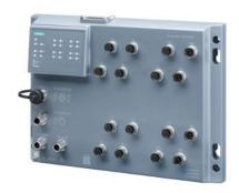
SCALANCE XP216, managed IE switch, 12x 10/100 Mbit/s IEC 62443-4-2 certified; M12 ports, 4x 10/100/1000 Mbit/s M12 ports IP65, LED diagnostics, error signaling contact, redundant power supply, PROFINET IO device, network management, can be operated in redundant ring, incl. dust caps, including electronic manual on CD-ROM, C-PLUG optional.
