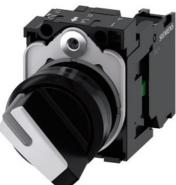
Selector switch, illuminable, 22 mm, round, plastic, white, selector switch, short, 2 switch positions O-I, latching, 10:30h/13:30h, with holder, 1 NO, screw terminal, with laser labeling, lower case
