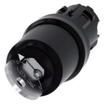
Key-operated switch IKON, 22 mm, round, plastic, lock number 360012K1, with 2 keys, 2 switch positions O-I, latching, actuating angle 90°, 10:30h/13:30h, key removal O, with laser labeling, inscription or symbol Customer-specific selection with SIRIUS ACT configurator (CIN)
