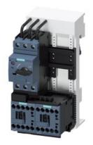
Load feeder fuseless, Reversing duty 400 V AC, Size S00 5.50...8.00 A 230 V AC screw terminal for 60 mm busbar systems Type of coordination 1, Iq = 150 kA 1 NC (contactor)
