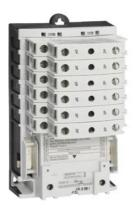
Electrically held lighting contactor, (convertible to mech. held), Amp rating 30A (tungsten 20A), 4 N.C. / 6 N.O. poles, 230-240V 60Hz/220V 50Hz coil, Noncombination type, Enclosure NEMA type (open), No enclosure
