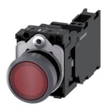
Illuminated pushbutton, 22 mm, round, plastic with metal front ring, red, pushbutton, flat, momentary contact type, with holder, 1 NO+1 NC, LED module with integrated LED 24 V AC/DC, spring-type terminal, with laser labeling, upper case and lower case, always upper case at beginning of line
