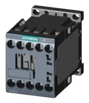
power contactor, AC-3, 16 A, 7.5 kW / 400 V, 4-pole, 110 V AC, 50 Hz / 120 V, 60 Hz, main contacts: 2 NO + 2 NC, screw terminal, size: S00
