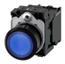
Illuminated pushbutton, 22 mm, round, plastic, blue, pushbutton, flat, momentary contact type, with holder, 1 NO, LED module with integrated LED 230 V AC, screw terminal
