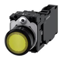
Illuminated pushbutton, 22 mm, round, plastic, yellow, pushbutton, flat, momentary contact type, with holder, 1 NO+1 NC, LED module with integrated LED 24 V AC/DC, screw terminal, with laser labeling, upper case
