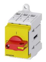
Load disconnector 3LD3, lu 32 A Main switch 3-pole Rated operating capacity for AC-23 A at 400V 11.5kW Installation in distribution boards, Basic switch with selector knob red / yellow
