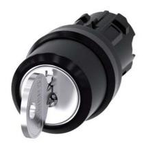
RONIS key-operated switch, 22 mm, round, plastic, lock number SB30, with 2 keys, 3 switch positions >O<II, momentary contact on the left, latching on the right, actuating angle  $2x45^\circ$ , 10:30h/12h/13:30h, key removal O, possible special locks: SB31, 421, 455 Z=50-unit packaging
