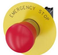
EMERGENCY STOP mushroom pushbutton, 22 mm, round, metal, shiny, red, 40 mm, positive latching, acc. to EN ISO 13850, pull-to-unlatch mechanism, with yellow backing plate, inscription: EMERGENCY STOP, with holder, 1 NC, screw terminal
