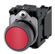
Pushbutton, 22 mm, round, plastic with metal front ring, red, pushbutton, flat, momentary contact type, with holder, 1 NO, screw terminal, with laser labeling, lower case
