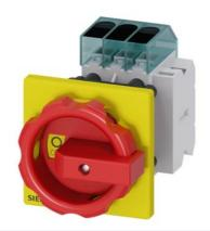
Load disconnector 3LD3, lu 32 A Main switch 3-pole Rated operating capacity for AC-23 A at 400V 11.5kW Front plate mounting Basic switch with Central hole mounting 22.5mm Rotary actuator red / yellow 66 x 66 mm with auxiliary switch 10E + 1S
