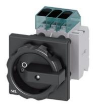
Load disconnector 3LD3, lu 32 A Main switch 3-pole Rated operating capacity for AC-23 A at 400V 11.5kW Front plate mounting Basic switch with Central hole mounting 22.5mm Rotating drive black 66 x 66 mm with auxiliary switch 1OE + 1S
