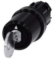
key-operated switch Siemens, 22 mm, round, plastic, lock number SSG10, with 2 keys, 3 switch positions I>O<II, momentary contact on the left, latching on the right, actuating angle 2x45°, 10:30h/12h/13:30h, key removal O, with laser labeling, upper case and lower case, always upper case at the beginning of the word
