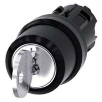
RONIS key-operated switch, 22 mm, round, plastic, lock number SB30, with 2 keys, 3 switch positions I>O<II, momentary contact on the left, latching on the right, actuating angle 2x45°, 10:30h/12h/13:30h, key removal O, possible special locks: SB31, 421, 455, with laser labeling, lower case
