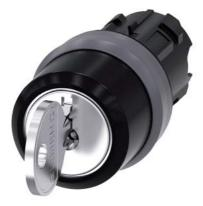
RONIS key-operated switch, 22 mm, round, plastic with metal front ring, lock number SB30, with 2 keys, 3 switch positions I>O<II, momentary contact on the left, latching on the right, actuating angle  $2x45^{\circ}$ , 10:30h/12h/13:30h, key removal O, possible special locks: SB31, 421, 455
