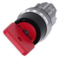
Key-operated switch O.M.R, 22 mm, round, metal, shiny, lock number 73037, red, with 2 keys, 2 switch positions O-I, latching, actuating angle  $90^\circ$ , 10:30h/13:30h, key removal O, with laser labeling, upper case and lower case, always upper case at the beginning of the word
