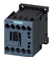
power contactor, AC-3e/AC-3, 9 A, 4 kW / 400 V, 3-pole, 110 V AC, 50 Hz / 120 V, 60 Hz, auxiliary contacts: 1 NO, screw terminal, size: S00
