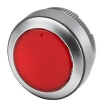
illuminated push-button for Extension Units, 22 mm, round, plastic, momentary contact type with integrated white LED, with 6 color filters (colorless, red, yellow, green, blue; black), 1 NO contact, without inscription (including printed-circuit board and contact module)
