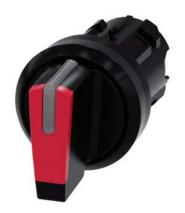
Selector switch, illuminable, 22 mm, round, plastic, red, selector switch, short, 3 switch positions I-O<II, left latching, right momentary contact type, actuating angle  $2x45^{\circ}$ , 10:30h/12h/13:30h
