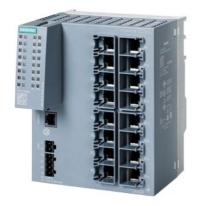
SCALANCE XC216EEC manageable Layer 2 IE switch; IEC 62443-4-2 certified; 16x 10/100 Mbit/s RJ45 ports; 1x console port; diagnostics LED; redundant power supply; with painted printed-circuit boards; NAMUR NE21-compliant; temperature range -40 °C to +70 °C; assembly: DIN rail/S7 mounting rail/wall redundancy functions; office features (RSTP, VLAN,...); PROFINET IO device; Ethernet/IPcompliant; C-PLUG slot;
