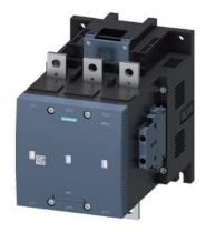
vacuum contactor AC-3e/AC-3 500 A, 250 kW / 400 V, 3-pole, Uc: 110-127 V AC(50-60 Hz) / DC drive: conventional auxiliary contacts 2 NO + 2 NC main circuit: busbar control and auxiliary circuit: screw terminal
