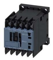
Coupling contactor relay, 2 NO + 2 NC, 24 V DC, 0.7  $\dots$  1.25\* US, with integrated suppressor diode, Size S00, Ring cable lug connection, suitable for PLC outputs
