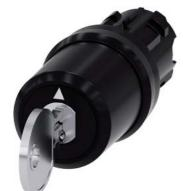
key-operated switch Siemens, 22 mm, round, plastic, lock number SSG10, with 2 keys, 3 switch positions I>O<II, momentary contact on the left, latching on the right, actuating angle 2x45°, 10:30h/12h/13:30h, key removal O, with laser labeling, inscription or symbol customer-specific selection with SIRIUS ACT configurator (CIN)
