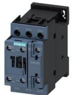
power contactor, AC-3e/AC-3, 9 A, 4 kW / 400 V, 3-pole, 480 V AC, 60 Hz, auxiliary contacts: 1 NO + 1 NC, screw terminal, size: S0
