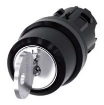
RONIS key-operated switch, 22 mm, round, plastic, lock number SB30, with 2 keys, 3 switch positions I-O-II, latching, actuating angle 2x45°, 10:30h/12h/13:30h, Key removal I+II, possible special locks: SB31, 421, 455, with laser labeling, upper case and lower case, always upper case at beginning of line
