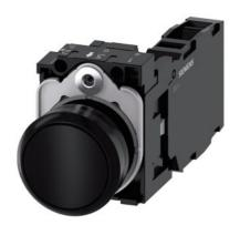
Pushbutton, 22 mm, round, plastic, black, pushbutton, flat, momentary contact type, with holder 1 NO+1 NC, screw terminal, with laser labeling, symbol number according to, ISO 7000 or IEC 60417
