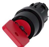
Key-operated switch O.M.R, 22 mm, round, plastic, lock number 73037, red, with 2 keys, 2 switch positions O-I, latching, actuating angle 90°, 10:30h/13:30h, key removal O, with laser labeling, inscription or symbol Customer-specific selection with SIRIUS ACT configurator (CIN)
