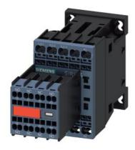
power contactor, AC-3e/AC-3, 12 A, 5.5 kW / 400 V, 3-pole, 110 V AC, 50 Hz / 120 V, 60 Hz, auxiliary contacts: 2 NO + 2 NC, spring-loaded terminal, size: S00, captive auxiliary switch
