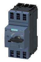
Circuit breaker size S00 for starter combination Rated current 1.6 A N-release 21 A Spring-type terminal Standard switching capacity
