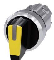
Selector switch, illuminable, 22 mm, round, metal, shiny, yellow, selector switch, short, 3 switch positions I>O<II, momentary contact type, actuating angle  $2x45^{\circ}$ , 10:30h/12h/13:30h
