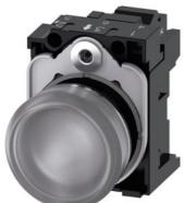
Indicator lights, 22 mm, round, metal, shiny, clear, lens, smooth, with holder, LED module with integrated LED 110 V AC, spring-type terminal, with laser labeling, upper case and lower case, always upper case at the beginning of the word
