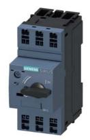
Circuit breaker size S00 for transformer protection A-release 2.2...3.2 A N release 65 A Spring-type terminal Standard switching capacity
