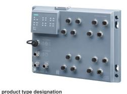
SCALANCE XP216EEC, managed IE switch, with railway approval IEC 62443-4-2 certified; (EN 50155, EN45545); 12x 10/100 Mbit/s M12 ports, 4x 10/100/1000 Mbit/s M12 ports IP65, LED diagnostics, error signaling contact, redundant power supply, PROFINET IO device, network management, can be operated in redundant ring, incl. dust caps, including electronic manual on CD-ROM, C-PLUG optional.
