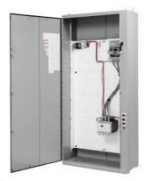
Enclosed soft starter, Controller 3RW44466BC34, Std duty rating 125HP @230V, Std duty current rating 315A Control voltage 115Vac Combination type, 600Amp fusible disconnect, Enclosure NEMA type 12, Dust/drip proof for indoors
