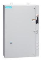
Non-reversing motor starter Size 0 Three phase full voltage Solid-state overload relay OLRelay amp range 0.75-3.4A 240V 50HZ / 277V 60HZ coil Combination type 3Amp circuit breaker Encl NEMA type 4X 316 S-steel Water/dust tight noncorrosive Extra-wide enclosure
