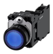
Illuminated pushbutton, 22 mm, round, plastic, blue, pushbutton, flat, momentary contact type, with holder, 1 NO+1 NC, LED module with integrated LED 230 V AC, spring-type terminal, with laser labeling, lower case
