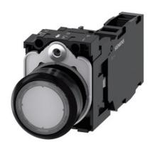
Illuminated pushbutton, 22 mm, round, plastic, clear, pushbutton, flat, momentary contact type, with holder, 1 NO+1 NC, LED module with integrated LED 230 V AC, screw terminal, with laser labeling, symbol number according to, ISO 7000 or IEC 60417
